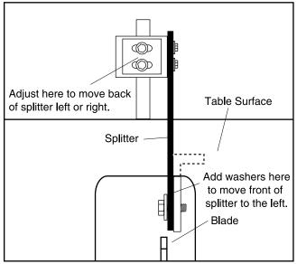
Figure 20. Improper splitter/blade alignment.
